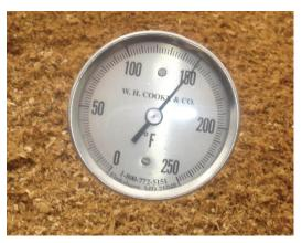
Figure 2. Long-stem thermometer used to monitor internal temperature. (credit: T. Guthrie.)
